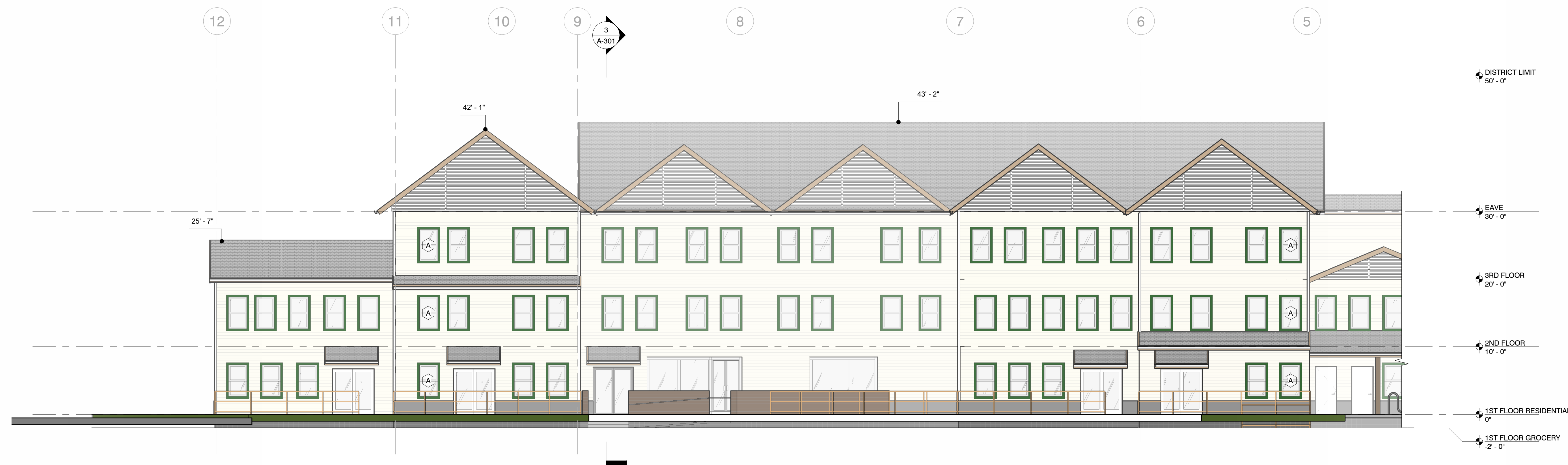
1 EXTERIOR WEST ELEVATION (RESIDENTIAL) SCALE: 1/8" = 1'-0"
